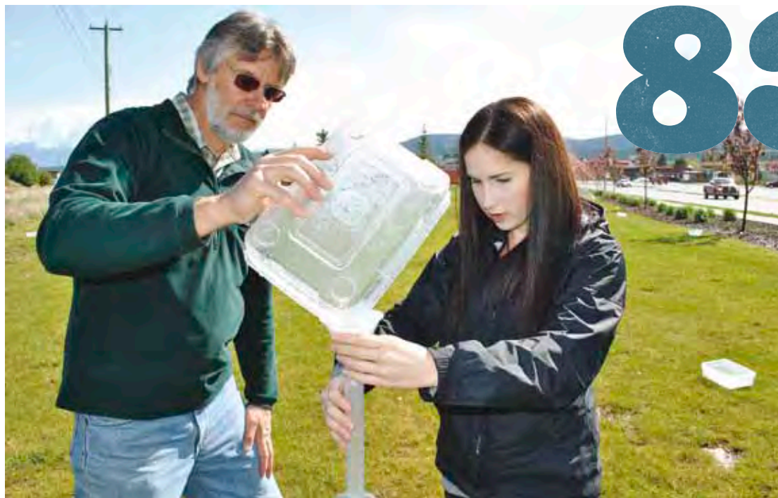
Water Smart Ambassadors determine the efficiency of an irrigation system by measuring the volume of water from the sprinklers. Find out if your community has a Water Smart Ambassador and call for your FREE lawn and garden water assessment.
